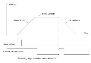
Figure 40: Home to Sensor (Go Forward To Next Sensor)
